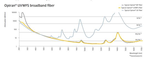
Optran® UVWFS fibers consist of an undoped core with a fluorine-doped jacket, with standard corejacket ratios of 1:1.06 and 1:1.4, as well as numerical apertures (NA) of 0.12 and 0.28. Customized designs are available upon request. The smallest bending radius amounts to 50 times the jacket or 300 times the core diameter. The protective polyimide jacket has a tensile strength of 70 kpsi (kilopound per square inch) and withstands temperatures from -190°C to up to +350°C.
