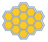
Bundles made from end-fused fibers show no gaps between individual fibers, since the fibers attain a hexagonal shape during the fusing process.
