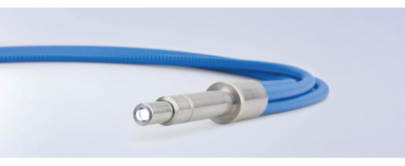
CeramOptec®'s fused-end PowerLightGuide bundles set the benchmark for consistently high long-term performance. The fusing process completely eliminates inter-fiber spaces and thus positions CeramOptec®'s PowerLightGuide bundles among the most sophisticated fiber bundles on the market. As the bundles do not rely on adhesive, they are resistant to temperatures of more than +600 °C, making them the first choice for demanding applications!
