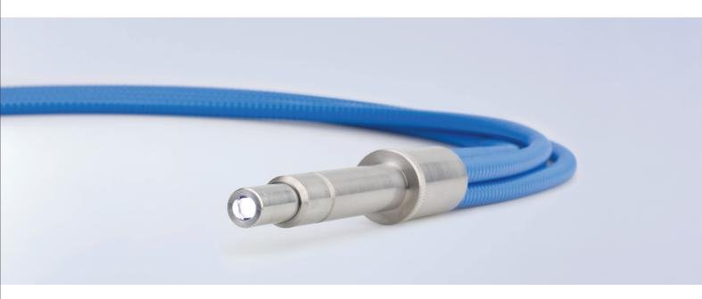
CeramOptec®'s fused-end bundles set the benchmark for consistently high long-term performance. The fusing process completely eliminates inter-fiber spaces and thus positions CeramOptec®'s fused-end bundles among the most sophisticated fiber bundles on the market. As the bundles do not rely on adhesive, they are resistant to temperatures of more than +600°C, making them the first choice for demanding applications!
